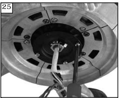
Loosen 3 screws with key slots and remove 1 screw without slot from motor plate and save screw.
